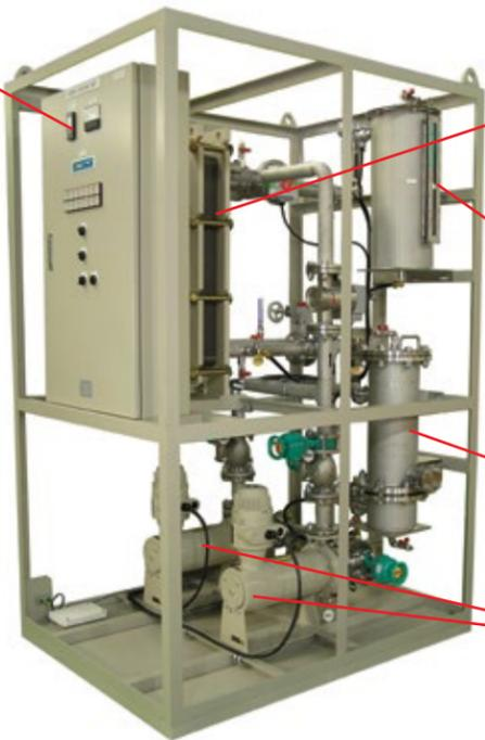
Water to water heat exchanger keeps the de-ionized system isolated from the plant water supply.
