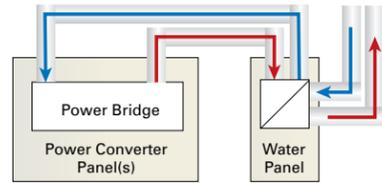
Separate type cooling has field-installed plumbing for de-ionized cooling loop.
