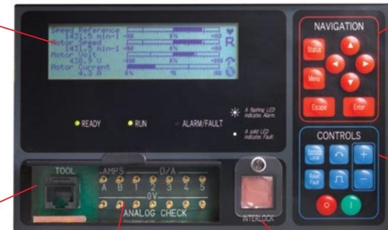
Easy-to-understand navigation buttons allow quick access to information without resorting to a PC-based tool
