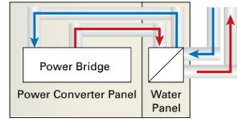
Integrated water system has internal plumbing for de-ionized cooling loop.
