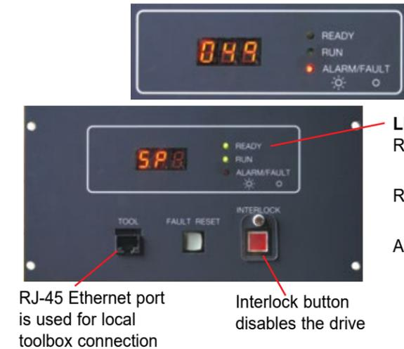
Three LEDs give a quick indication of the status of the unit
