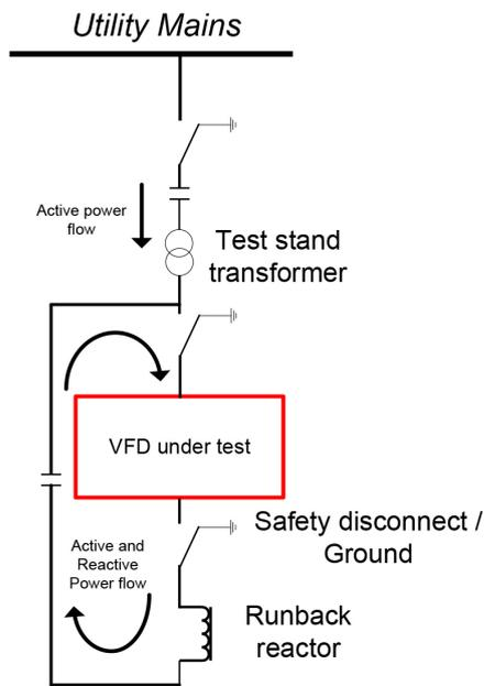
**Figure 3.** Runback reactor test set-up. © 2017 IEEE. Reprinted with permission.<sup>1</sup>
