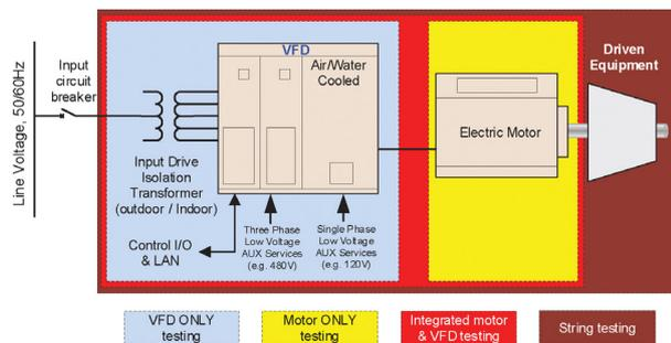
**Figure 1.** Typical large VFD and motor configuration. © 2017 IEEE. Reprinted with permission.<sup>1</sup>
