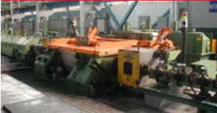
TMEIC's looperless minimum tension control is obtained by measuring torque and controlling stand speed, with upstream stands under cascade control. The automation system tracks billets from the furnace, through the rolling stands, cooling bed, no-twist block and shears to the finished coils. Product data is sent to each stage controls and HMIs.
