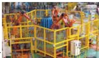
*Robotic Stator Core Lamination Stacking*
