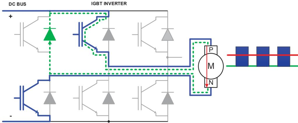
Figure 2, DC Motor Armature Positive Voltage case (Quadrant 1)<sup>1</sup>
