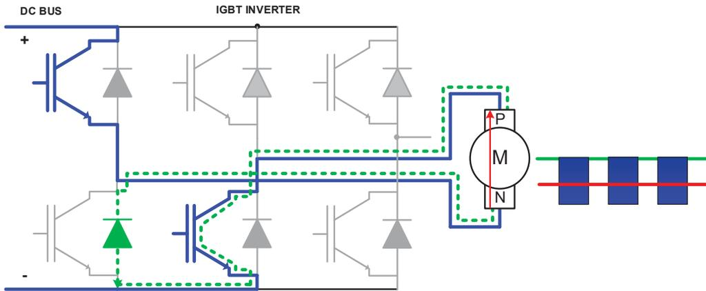
Figure 3, DC Motor Armature Negative Voltage case (Quadrant 3)<sup>1</sup>
