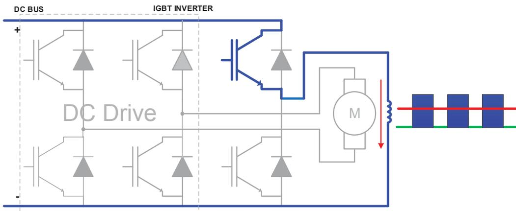
Figure 4, Inverter Bridge provides excitation for DC Motor Field<sup>1</sup>
