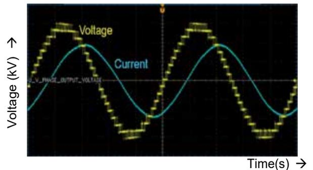
\*Example of the actual test result of the standard 4.16 kV VFD
