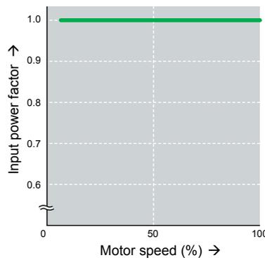
Example of the actual load test result of the standard 4-pole motor
