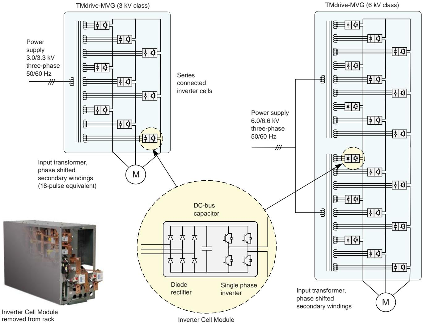
Inside the TMdrive-MVG Cabinet – an example of the 6 kV class drive with inverter cell detail.
