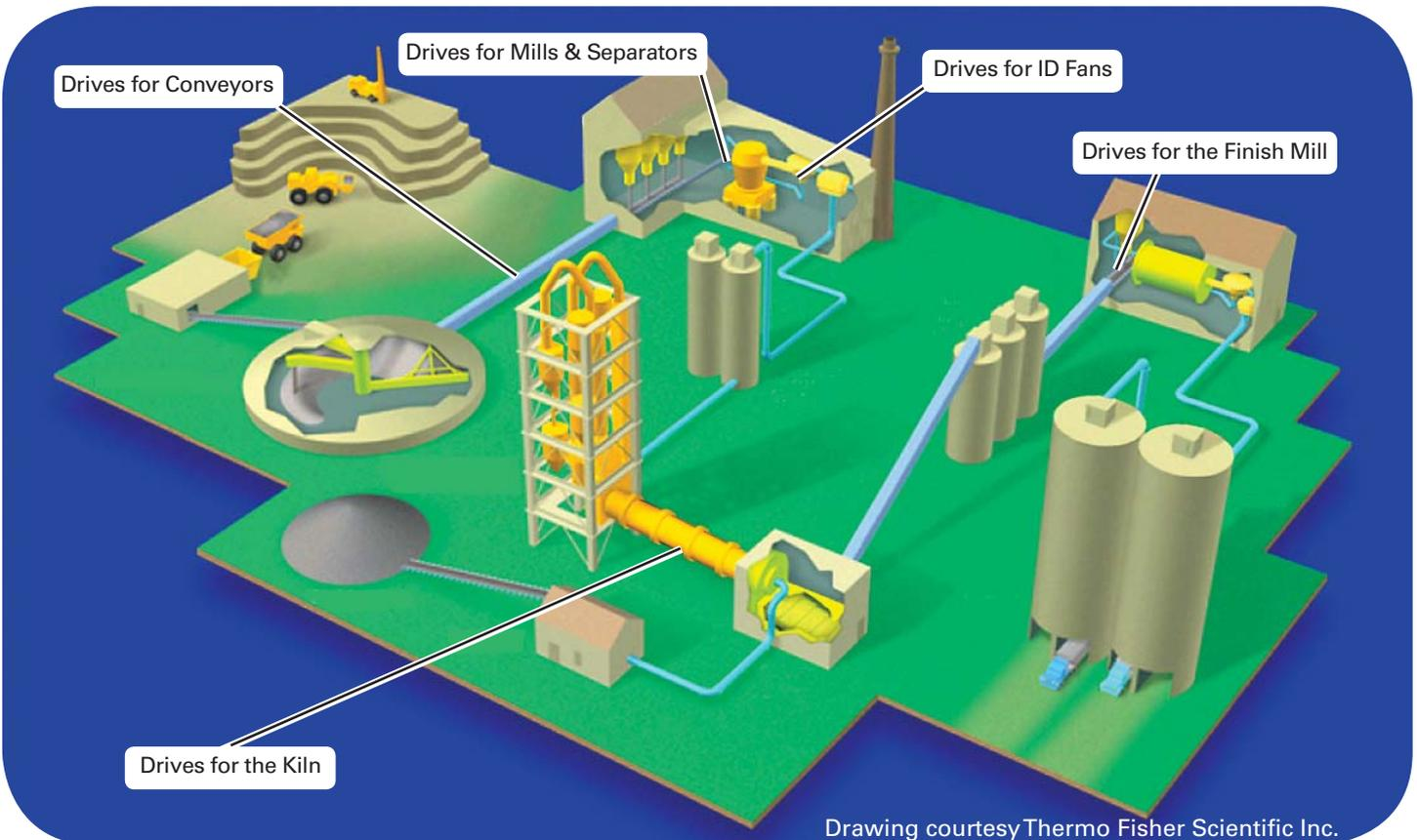
Controlling fan flow by adjusting speed avoids wasting energy in adjustable dampers and louvers. When large flows are involved and the motor energy consumption is significant, varying the speed is the answer. With large
