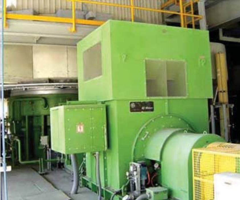
Synchronous Motor for Mill
