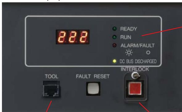
RJ-45 Ethernet port is used for local tool connection
