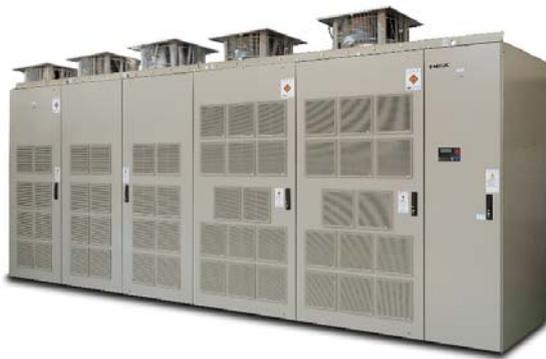
The TMdrive-MVG is a general-purpose, medium-voltage, variable-frequency AC drive for industrial power ratings up to 10 MW, in the voltage range of 3/3.3 kV, 6/6.6 kV and 10/11 kV.
