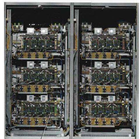
TM-70 10MVA Converter 10 MVA Inverter
