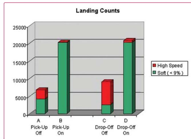
Figure 4. Total landing count of container pick-ups and drop-offs, with the smart landing system on and off.
