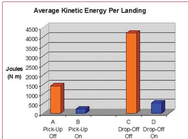
Figure 5. Average kinetic energy per landing for container pick-ups and drop-offs, with the smart landing system on and off.
